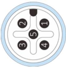
Figure 17: M12 Pin definition(sensor side)
