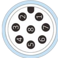
Figure 14: M12 8 Pin definition(sensor side)
