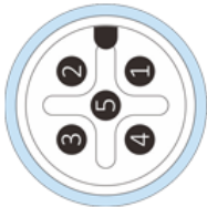
Figure 15: M12 Pin definition(sensor side)
