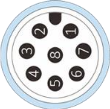
Figure 16: M12 Pin definition(sensor side)
