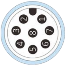
Figure 18: M12 Pin definition(sensor side)
