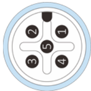
Figure 13: M12 5 Pin definition(sensor side)
