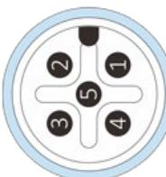
**Figure 14: M12 Pin definition(sensor side)****Table 18: CAN pin description**
