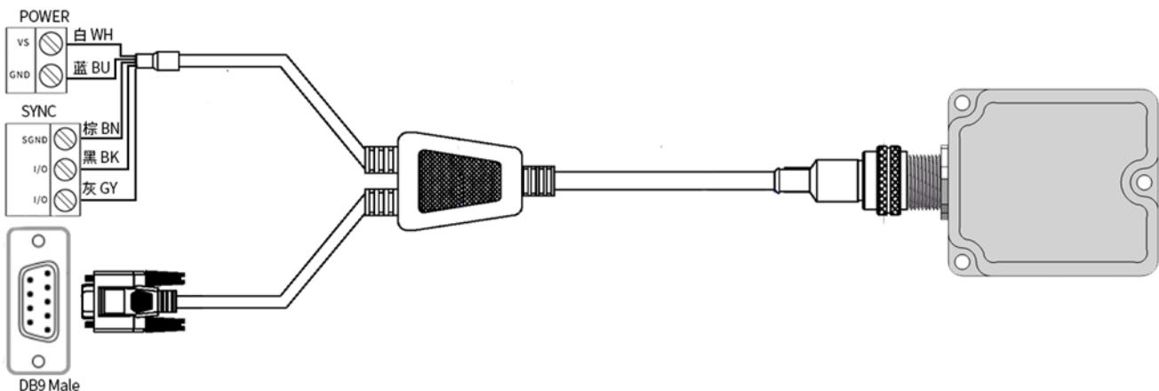
Figure 17: M12-A code 8pin to DB9+OPEN external power
