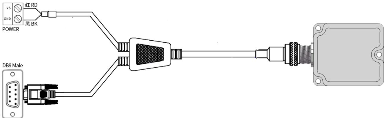
Figure 16: M12-A code 5pin to DB9+OPEN external power
