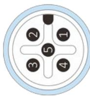
**Figure 13: M12 Pin definition(sensor side)****Table 17: RS-485 pin description**
