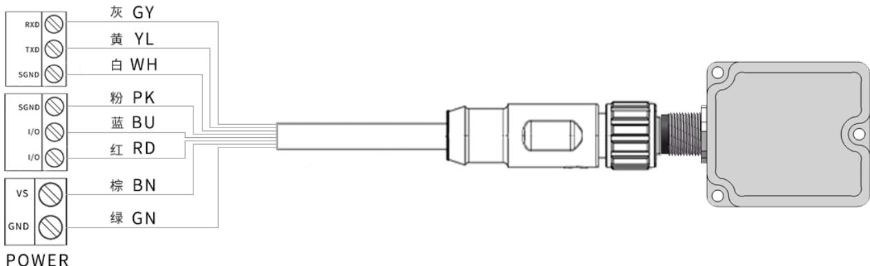
Figure 24: Synchronous with UART not common ground
