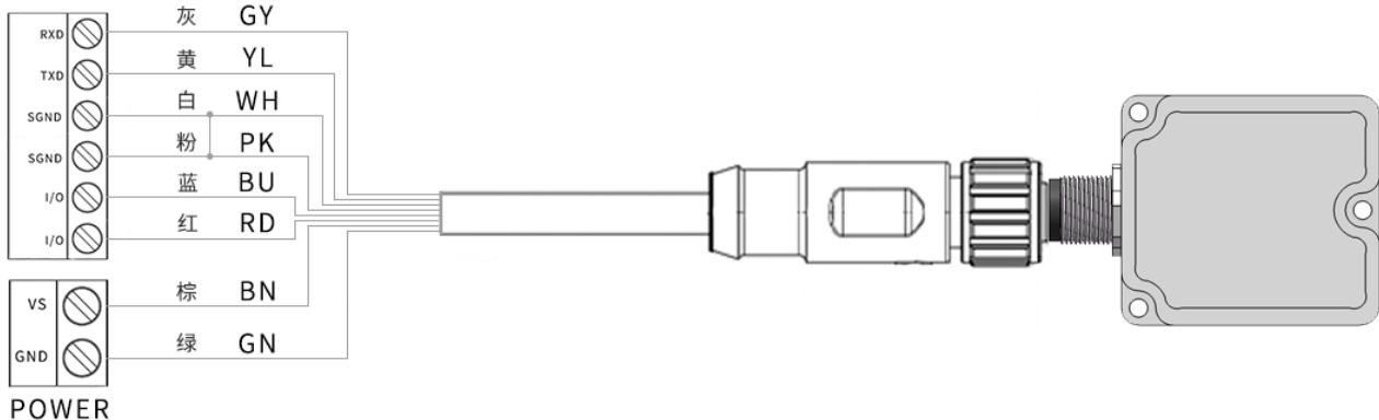
Figure 23: Synchronous with UART common ground
