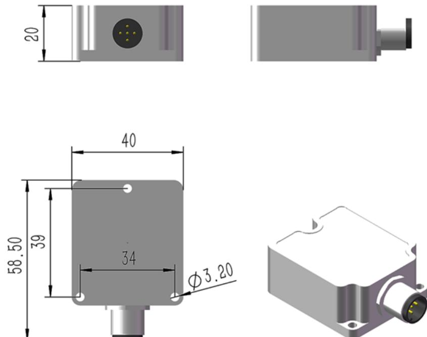
Figure 10: HI14 M12 Mechanical Dimension
