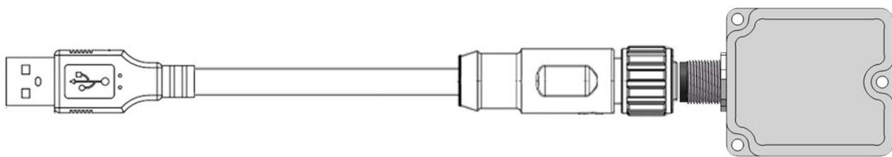
Figure 19: M12-A code 5pin to USB A
