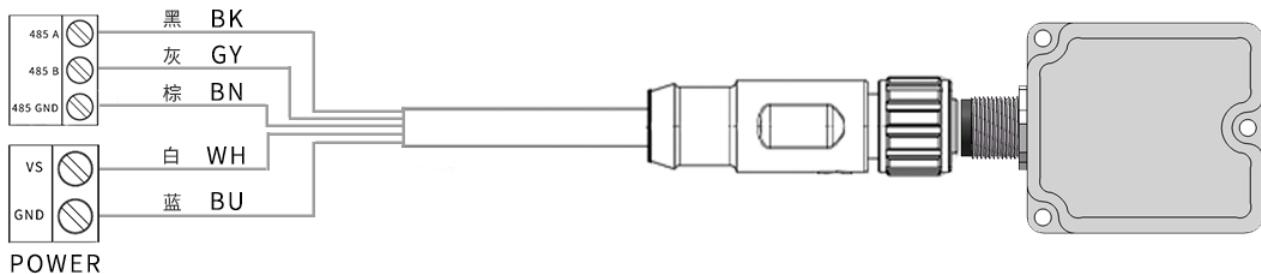
Figure 20: M12-A code 5pin to open RS-485
