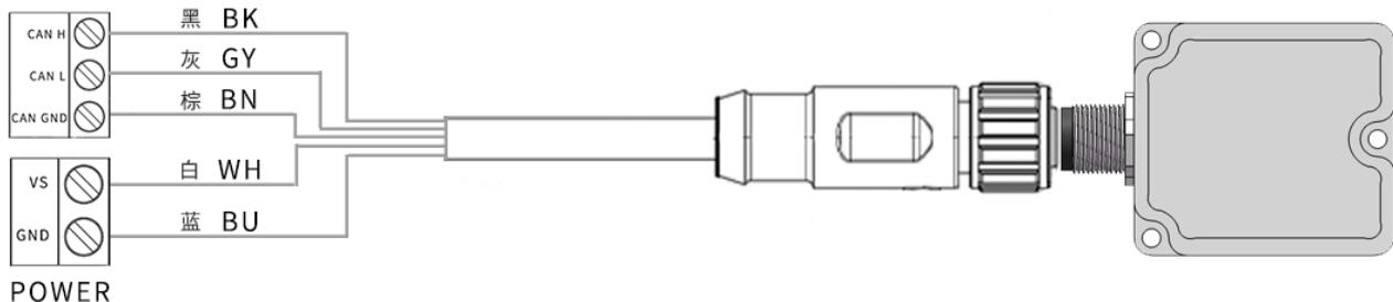
Figure 21: M12-A code 5pin to open CAN
