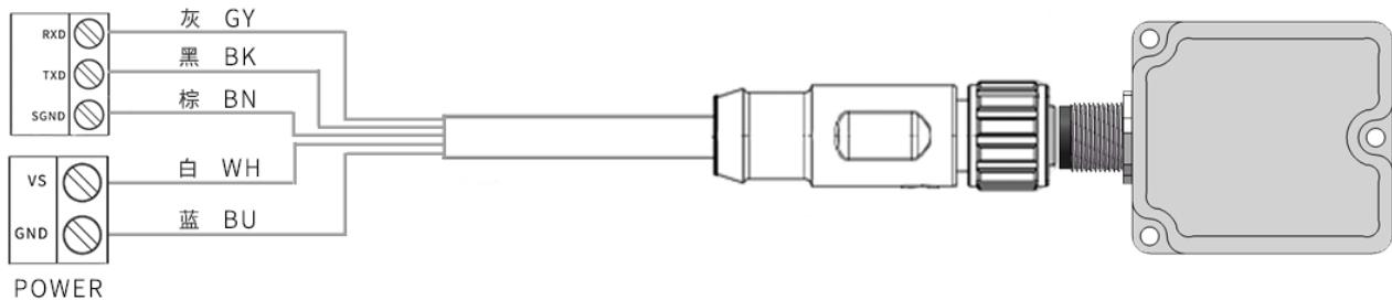
Figure 22: M12-A Code 5pin to Open UART
