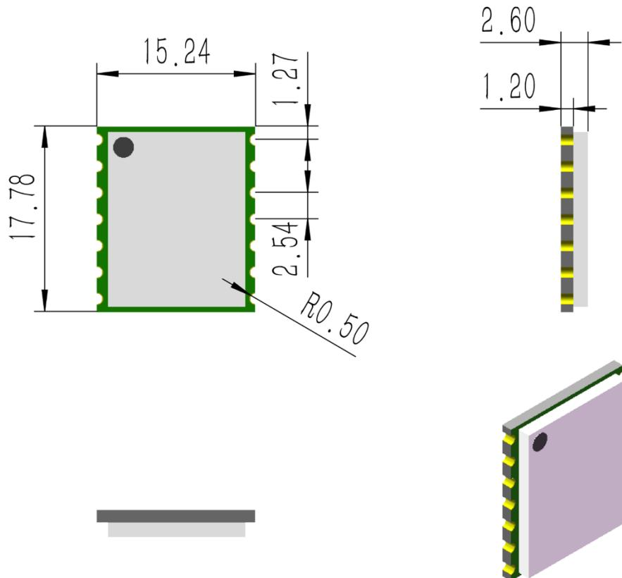
Figure10: CH010/CH020 Mechanical Dimension
