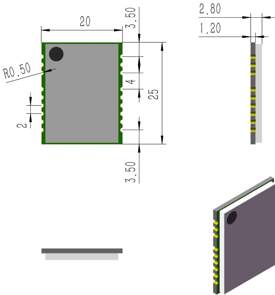
Figure12: CH040/CH040MP Mechanical Dimension
