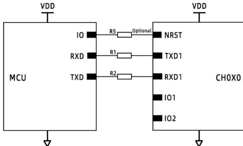
Figure17: *CH0X0 Serial Communication Reference Circuit Diagram*
