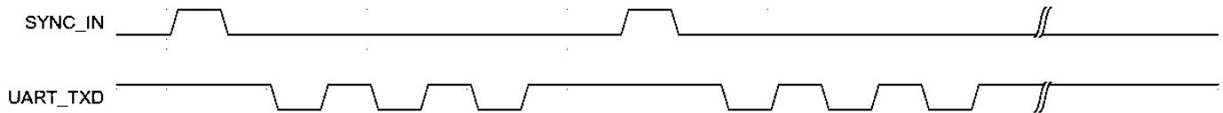
Figure22: Sync\_In Timing
