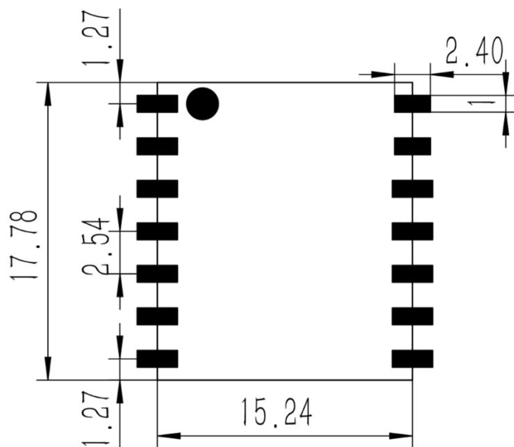
Figure11: CH010/CH020 Recommended Footprint
