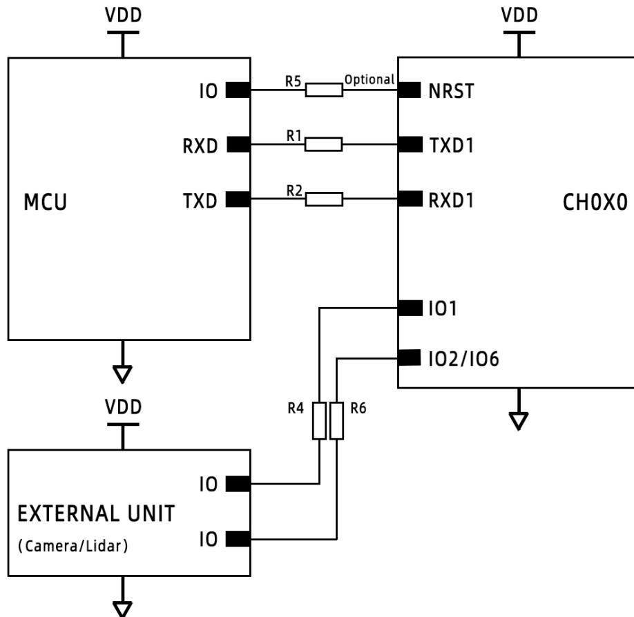
Figure20: *CH0X0 Serial Communication with External System Synchronization 2*
