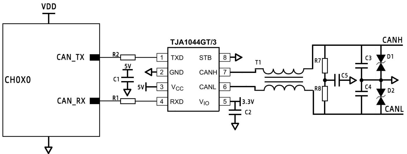
Figure21: CH0X0 series CAN communication circuit reference
