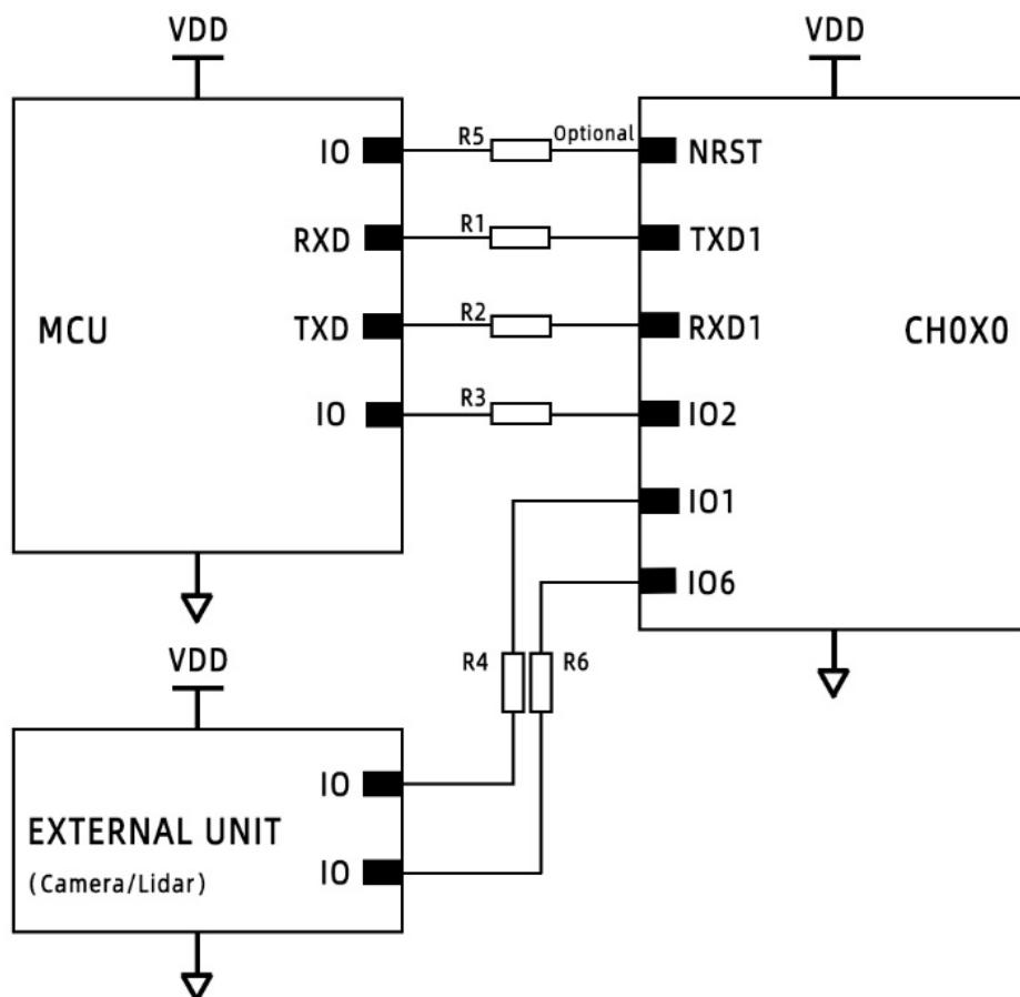
Figure19: CH0X0 Serial Communication with External System Synchronization 1
