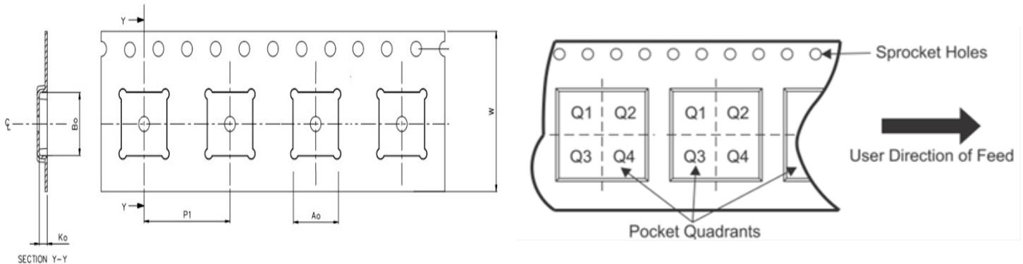
Figure26: Tape Dimension and pin 1
