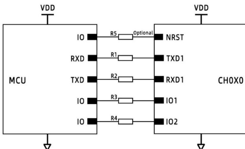
Figure18: *CH0X0 Serial Communication with Synchronization*
