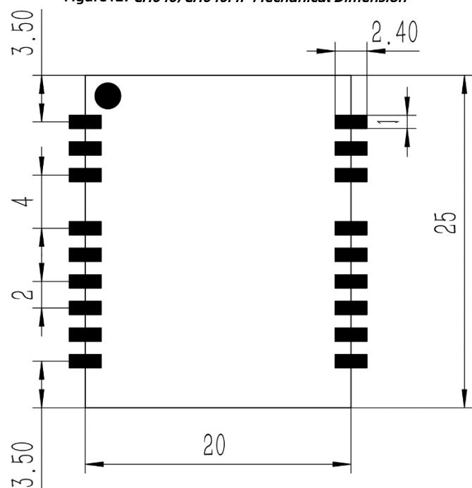
Figure13: CH040/CH040MP Recommended Footprint
