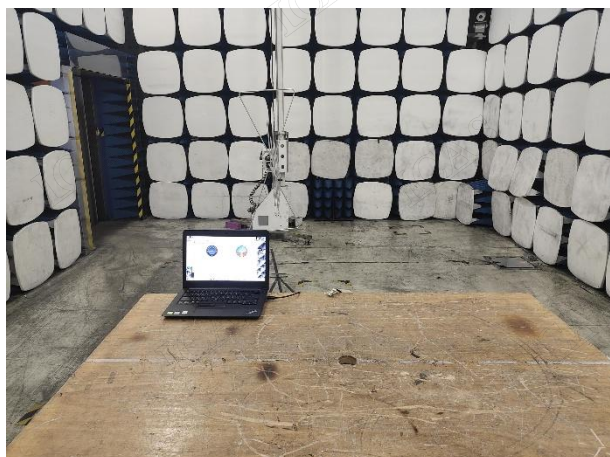
Electrostatic Discharges Test Set-up
