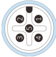
Figure 3: HI14 M12 5-Pin A-Coded Male Connector Pin Numbering
