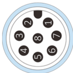
Figure 4: HI14 M12 A-Coded Male Connector Pin Numbering
